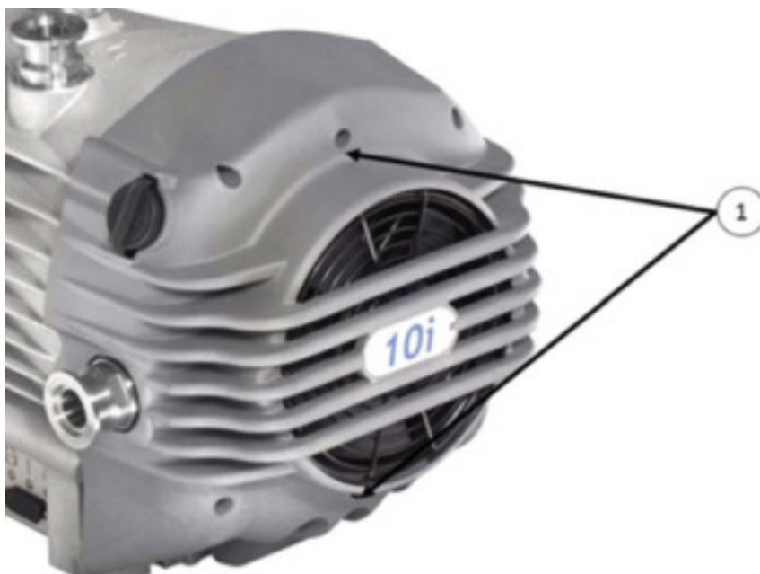
Figure 1 - Fan cowl removal
